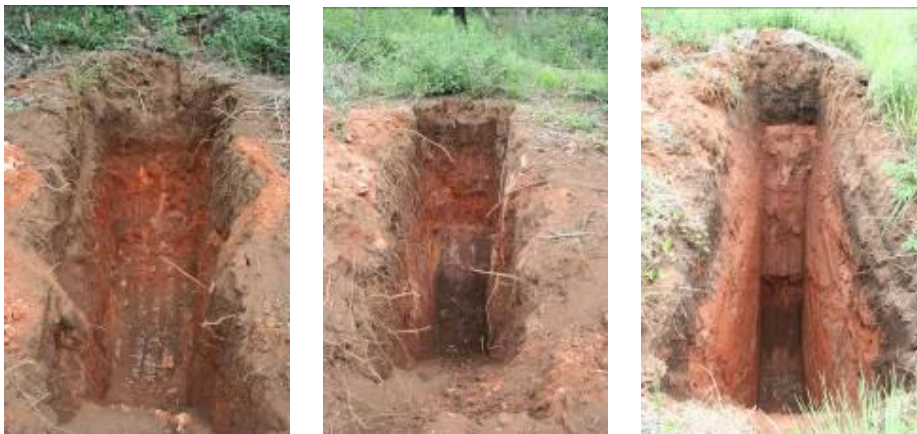
Fig 1. Test pits dug on-site to determine the depth and structure of the soil.
