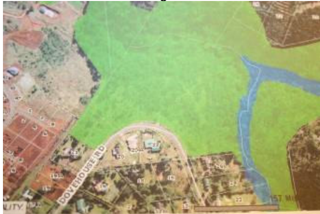
Fig 4: The green shadowed area is D'MOSS, the blue shaded area is within the 1 in 100 year flood line
